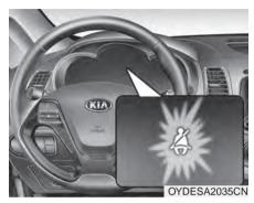
As a reminder to the driver, the driver's seat belt warning lights will illuminate for approximately 6 seconds each time you turn the ignition switch ON regardless of belt fastening. If the driver's seat belt is not fastened when the ignition switch is turned ON or if it is disconnected after the ignition switch is turned ON, the seat belt warning light will illuminate until the belt is fastened.
