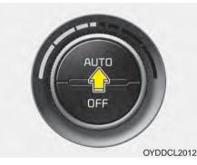
1. Push the AUTO button. The modes, fan speeds, air intake and air-conditioning will be controlled automatically by temperature setting. Driver's side
