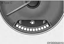
The fuel gauge indicates the approximate amount of fuel remaining in the fuel tank. The fuel tank capacity is given in chapter 8. The fuel gauge is supplemented by a low fuel warning light, which will illuminate when the fuel tank is nearly empty. On inclines or curves, the fuel gauge pointer may fluctuate or the low fuel warning light may come on earlier than usual due to the movement of fuel in the tank.
