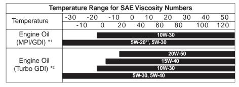
\*1. For better fuel economy, it is recommended to use the engine oil of a viscosity grade SAE 5W-20 (API SM / ILSAC GF-4). However, if the engine oil is not available in your country, select the proper engine oil using the engine oil viscosity chart.
