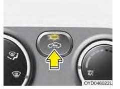
This is used to select outside (fresh) air position or recirculated air position. To change the air intake control position, push the control button.
