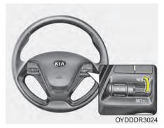
If any method other than the CRUISE button was used to cancel cruising speed and the system is still activated, the most recent set speed will automatically resume when you move the lever up (to RES+).
