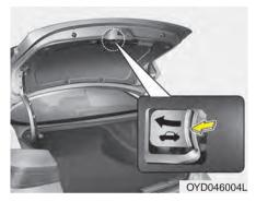
Your vehicle is equipped with an emergency trunk release lever located inside the trunk. If someone is inadvertently locked in the trunk, moving the handle in the direction of the arrow will release the trunk latch mechanism and open the. No one should be allowed to occupy the trunk at any time. The trunk is a very dangerous location in the event of a crash.
