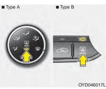
The defroster heats the window to remove frost, fog and thin ice from the interior and exterior of the rear window, while the engine is running.
