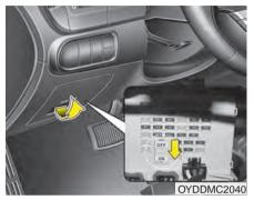
Your vehicle is equipped with a fuse switch to prevent battery discharge if your vehicle is parked without being operated for prolonged periods.
