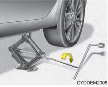
8. Insert the jack handle into the jack and turn it clockwise, raising the vehicle until the tire just clears the ground. This measurement is approximately 1 in (30 mm). Before removing the wheel lug nuts, make sure the vehicle is stable and that there is no chance for movement or slippage. 9. Loosen the wheel nuts and remove
