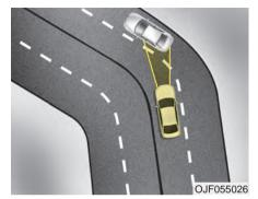
While driving on a curve, the AEB may recognize the vehicle in front in the next lane. Exercise caution, and, if necessary, depress the brake pedal.
