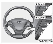
The LCD window modes can be changed by using the control buttons on the steering wheel.
