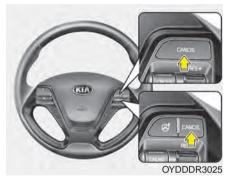
Each of these actions will cancel cruise control operation (the SET indicator light in the instrument cluster will go off), but it will not turn the system off. If you wish to resume cruise control operation, move up the lever (to RES+) located on your steering wheel. You will return to your previously preset speed.
