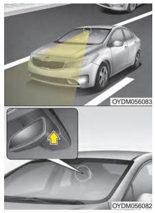
The Lane Keeping Assist System detects lane markers on the road, and assists the driver's steering to help keep the vehicle between lanes. When the system detects the vehicle straying from its lane, it alerts the driver with a visual and audible warning, while applying a slight countersteering torque, trying to prevent the vehicle from moving out of its lane.
