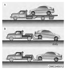
If emergency towing is necessary, we recommend having it done by an authorized Kia dealer or a commercial tow-truck service. Proper lifting and towing procedures are necessary to prevent damage to the vehicle. The use of wheel dollies or flatbed is recommended. It is acceptable to tow the vehicle with the rear wheels on the ground (without dollies) and the front wheels off the ground.
