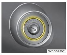
Whenever a front door is opened, the ignition switch will illuminate for your convenience, provided the ignition switch is not in the ON position. The light will go off immediately when the ignition switch is turned on. It will also go off after about 30 seconds after the door is closed.
