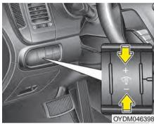
The instrument panel illumination intensity can be adjusted by pressing the control switch with the headlight switch in any position when the ignition switch is in the ON position.
