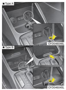
The power outlet is designed to provide power for mobile telephones or other devices designed to operate with vehicle electrical systems. The devices should draw less than 12V, 15A with the engine running. Use the power outlet only when the engine is running and remove the accessory plug after use. Using the accessory plug for prolonged periods of time with the engine off could cause the battery to discharge.
