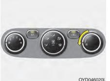
The MAX A/C mode is used to cool the inside of the vehicle faster. Air flow is directed toward the upper body and face.
