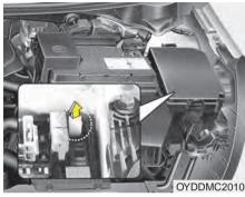
If the headlights or other electrical components do not work and the fuses are OK, check the fuse panel in the engine compartment. If a fuse is blown, it must be replaced.
