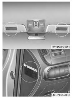
Air bag warning labels, some required by the U.S. National Highway Traffic Safety Administration (NHTSA), are attached to alert the driver and passengers of potential risks of the air bag system.
