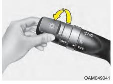
When the light switch is in the parking light position (1st position), the tail, position, license and instrument panel lights will turn ON.
