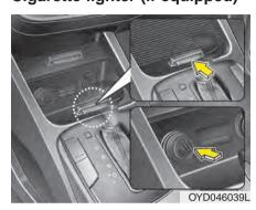
For the cigarette lighter to work, the ignition switch must be in the ACC or ON position.
