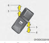
Pressing or pulling up the power window switch momentarily to the second detent position (6) completely lowers or lifts the window even when the switch is released. To stop the window at the desired position while the window is in operation, pull up or press and release the switch to the opposite direction of the movement.
