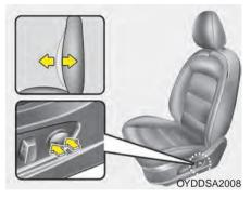
The lumbar support can be adjusted by pressing the lumbar support switch on the side of the driver's seat. Press the front portion of the switch to increase support, or the rear portion of the switch to decrease support. Driver position memory system (if equipped, for power seat)
