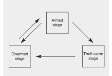
This system is designed to provide protection from unauthorized entry into the vehicle. This system is operated in three stages: the first is the "Armed" stage, the second is the "Theft-alarm" stage, and the third is the "Disarmed" stage. If triggered, the system provides an audible alarm with blinking of the hazard warning lights.
