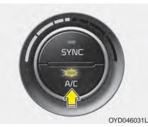
Press the A/C button to turn the air conditioning system on (indicator light will illuminate).
