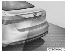
Always keep the camera lens clean. If lens is covered with foreign matter, the camera may not operate normally.
