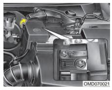
Visually inspect the battery cap to ensure it is securely closed. If the battery cap is not securely closed, moisture may enter the system and damage the electrical components.
