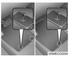
When using a floor mat on the floor carpet, make sure it attaches to the floor mat anchor(s) in the front and rear floor carpet of your vehicle. This keeps the floor mat from sliding forward.
