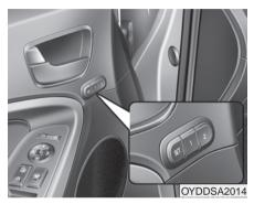
A driver position memory system is provided to store and recall the driver seat position with a simple button operation. By saving the desired position into the system memory, different drivers can reposition the driver seat based upon their driving preference. If the battery is disconnected, the desired seat position memory will need to be re-saved. WARNING - Driver position memory system
