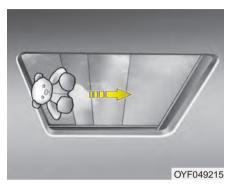
If an object or part of the body is detected while the sunroof glass or sunshade is closing automatically, it will reverse the direction, and then stop.
