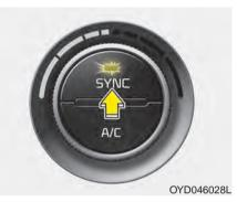
Adjusting the driver and passenger side temperature individually
