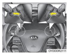
The paddle shifter is available when the shift lever is in the D (Drive) position or the manual mode. With the shift lever in the D position
