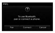
If *Bluetooth*<sup>®</sup> Wireless Technology devices are paired but none are currently connected, pressing the [PHONE] button or the [CALL] button on the steering wheel control displays the following screen. Press the [Pair] to pair a new device or press the [Connect] to connect a previously paired device. *Pairing through [PHONE] Setup* Press the **[SETUP]** button ► Select [Phone].
