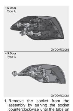
the socket align with the slots on
