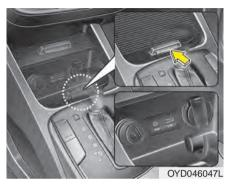
If your vehicle has an aux and/or USB(universal serial bus) port or iPod<sup>®</sup> port, you can use an aux port to connect audio devices and an USB port to plug in an USB and also an iPod<sup>®</sup> port to plug in an iPod<sup>®</sup>.
