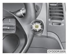
Whenever the front door is opened, the ENGINE START/STOP button will illuminate for your convenience. The light will go off after about 30 seconds after the door is closed. ENGINE START/STOP button position
