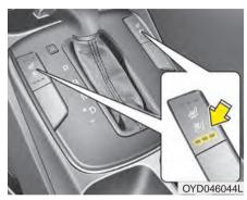
The climate control seat is provided to cool or warm the seat during hot or cold weather by blowing air through small vent holes on the surface of the seat and seatback. While the engine is running, push the rear portion of the switch (blue color) to cool the seat, and push the front portion of the switch (red color) to warm the seat.
