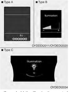
• If you hold the illumination control button ("+" or "-"), the brightness will be changed continuously.
