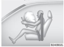
Upon deployment, tear seams molded directly into the pad covers will separate under pressure from the expansion of the air bags. Further opening of the covers then allows full inflation of the air bags. Driver's front air bag (3)
