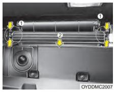
3. Remove the climate control air filter case by pulling out both sides of the cover.
