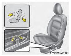
Push the control switch forward or backward to move the seatback to the desired angle. Release the switch once the seat reaches the desired position.
