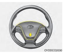
To sound the horn, press the horn symbol on your steering wheel. Check the horn regularly to be sure it operates properly.
