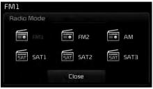
Pressing the **[RADIO]** button will change the operating mode in the order of FM1  $\rightarrow$  FM2  $\rightarrow$  AM  $\rightarrow$  SAT1  $\rightarrow$  SAT2  $\rightarrow$  SAT3.
