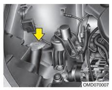
Check the fluid level in the washer fluid reservoir and add fluid if necessary. Plain water may be used if washer fluid is not available. However, use washer solvent with antifreeze characteristics in cold climates to prevent freezing.
