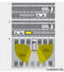
The Blind Spot Detection System (BSD) uses a radar sensor to alert the driver.
