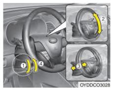
To change the steering wheel angle, pull down the lock release lever (1), adjust the steering wheel to the desired angle (2) and height (3), then pull up the lock-release lever to lock (4) the steering wheel in place. Be sure to adjust the steering wheel to the desired position before driving. Horn
