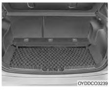
To keep items from shifting in the cargo area, you can use the four holders located in the cargo area to attach the luggage net.
