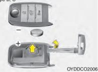
A battery should last for several years, but if the transmitter or smart key is not working properly, try replacing the battery with a new one. If you are unsure how to use or replace the battery, contact an authorized Kia dealer.
