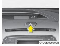
The hazard warning flasher serves as a warning to other drivers to exercise extreme caution when approaching, overtaking, or passing your vehicle. It should be used whenever emergency repairs are being made or when the vehicle is stopped near the edge of a roadway.
