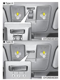
Push the lens (1) to turn the map lamp on or off. This light produces a spot beam for convenient use as a map lamp at night or as a personal lamp for the driver and front passenger.
