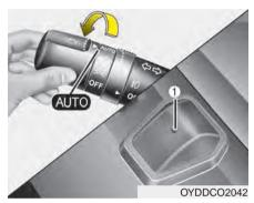
Never place anything over the sensor(1) located on the instrument panel. This will ensure better autolight system to turn on and off automatically.
