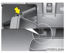
Auto defogging reduces the probability of fogging up the inside of the windshield by automatically sensing the moisture inside the windshield.
