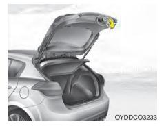
To close the tailgate, lower and push down the tailgate firmly. Make sure that the tailgate is securely latched.
