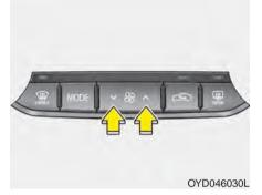
The fan speed can be set to the desired speed by pressing the fan speed control switch.
