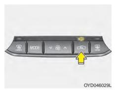
The air intake control is used to select outside (fresh) air position or recirculated air position.
