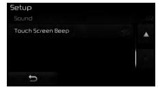
**Touch Screen Beep** This feature is used to turn the touch screen beep on/off.
