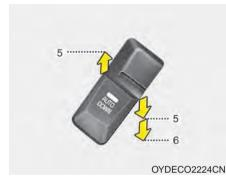
Pressing the power window switch momentarily to the second detent position (6) completely lowers the driver's window even when the switch is released. To stop the window at the desired position while the window is in operation, momentarily pull up the switch to the opposite direction of the window movement. Auto up/down window (if equipped)
