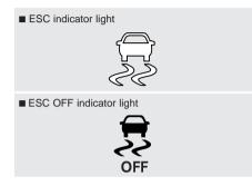
When the ignition switch is turned ON, the indicator light illuminates, then goes off if ESC system is operating normally.
