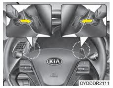
The paddle shifter is available when the shift lever is in the D position or the sport mode.
