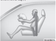
The air bag modules are located both in the center of the steering wheel and in the front passenger's panel above the glove box. When the SRSCM detects a sufficiently severe impact to the front of the vehicle, it will automatically deploy the front air bags. Driver's front air bag (2)
