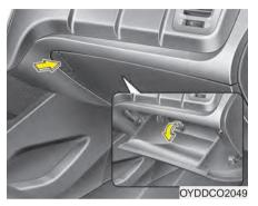
To open the glove box, push the button (1) and the glove box will automatically open. Close the glove box after use.
