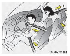
Your vehicle is equipped with driver's and front passenger's pre-tensioner seat belts.
