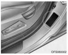
The vehicle certification label attatched on the driver's side center pillar gives the vehicle identification number (VIN).
