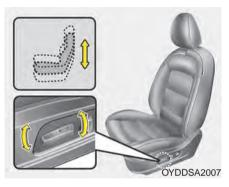
Pull the front portion of the control switch up to raise or down to lower the front part of the seat cushion. Pull the rear portion of the control switch up to raise or down to lower the rear part of the seat cushion. Release the switch once the seat reaches the desired position.
