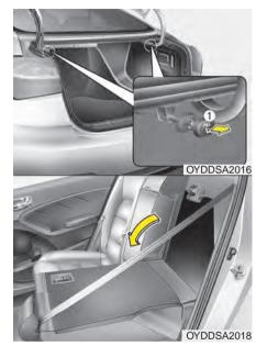
5.Pull the lock release lever (1) and fold the rear seatback forward and down firmly.
