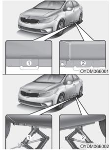
7.Place the jack at the front or rear jacking position closest to the tire you are changing. Place the jack at the designated locations under the frame. The jacking positions are plates welded to the frame with two tabs and a raised dot to index with the jack. A WARNING - Jack location
