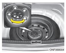
Turn the tire hold-down wing bolt counterclockwise.
