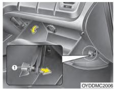
1. Open the glove box and pull the support strap (1).
